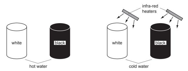
The hot water in the black can cools more quickly than the hot water in the white can. The cold water in the black can heats up more quickly than the cold water in the white can.
