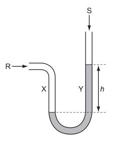
Side X is connected to a gas supply. Side Y is open to the atmosphere.
