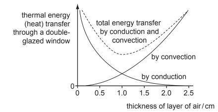
Which thickness of air produces the smallest energy transfer, and why?
