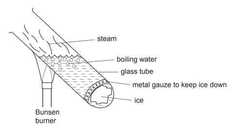
Why does the ice take a long time to melt, even though the water at the top of the tube is boiling?
