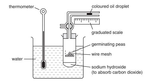
22 The diagram shows apparatus used to investigate respiration.
